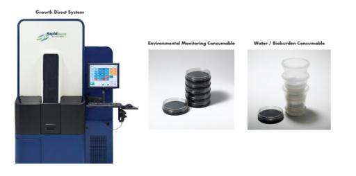
Our Growth Direct system is a fully automated, high throughput instrument for daily processing of MQC samples on our consumables — a microbiology quality control lab in a box. The Growth Direct system contains two high-capacity incubators, an advanced imaging system and internal robotics for sample handling. The system enables walk-away bulk sample loading, holding 700 of our consumables per instrument. Its dual, independently
