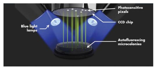
Illumination of a sample via a blue LED light causes microcolonies to fluoresce
