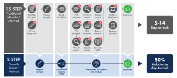
Our Growth Direct platform accelerates time to results by several days, a 50% improvement over the traditional method, and reduces MQC testing to a simple two-step workflow, eliminating 85% of the manual steps of traditional MQC, generating significant time, operational, and cost savings for our customers.
