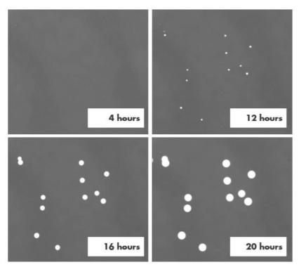
A key feature of detection via imaging of autofluorescence is that this approach does not harm cells, and as such is a non-destructive method. This provides several benefits, including ensuring that detected colonies represent actual viable microbial contaminations, and permitting detected microcolonies to grow into visible colonies for use in subsequent microbial identification for root cause investigation follow-up.
